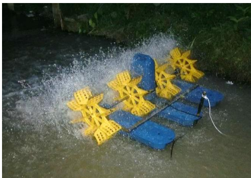
Figure 12. Working paddle-wheel aerator connected to the inverter
