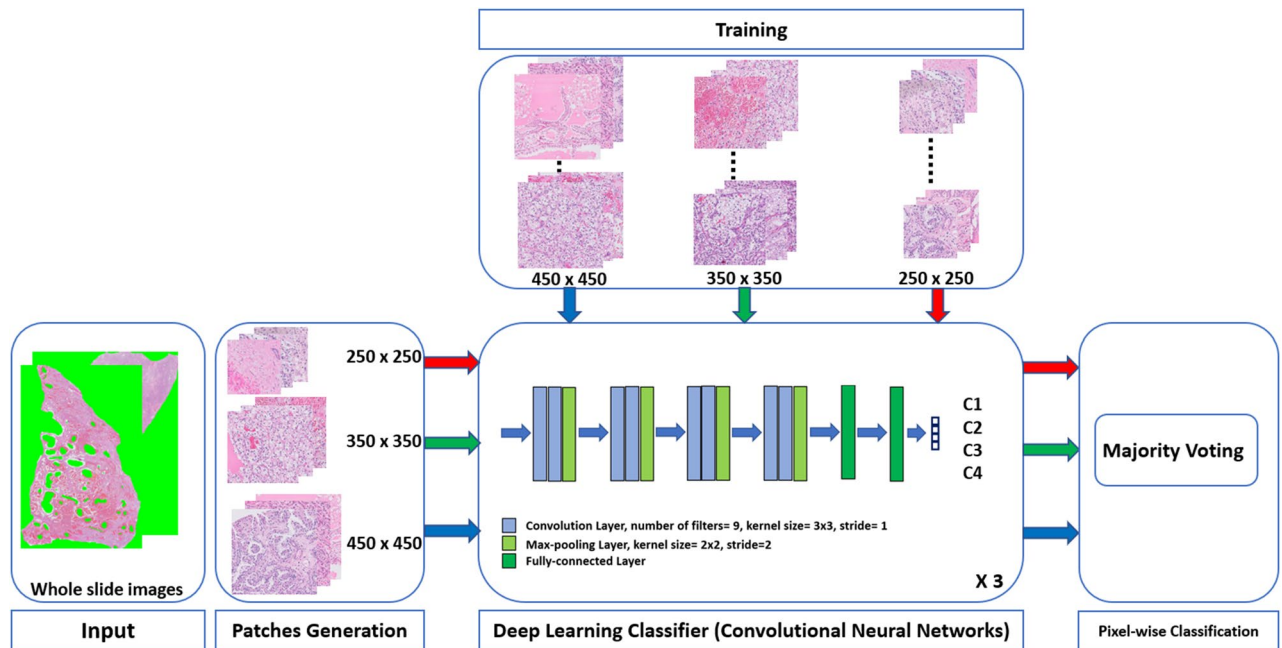
Figure 1. Schematic illustration of the proposed computer aided diagnostic system for automated classification of kidney tissues.
