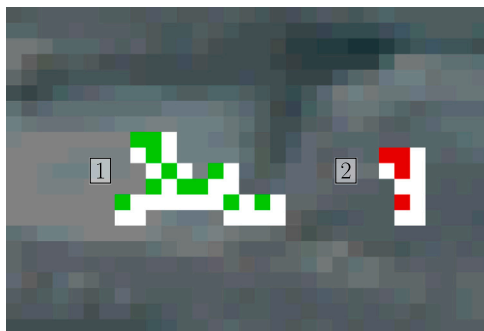
Fig. 5. Selection of connected components. The detected regions are dilated by one pixel on the right and on the bottom (white regions). Region 1 contains more than 5 detected pixels (11, in green) and thus it is selected; region 2 contains less than 5 detected pixels (4, in red) and thus it is discarded. (For interpretation of the references to color in this figure legend, the reader is referred to the web version of this article.)
