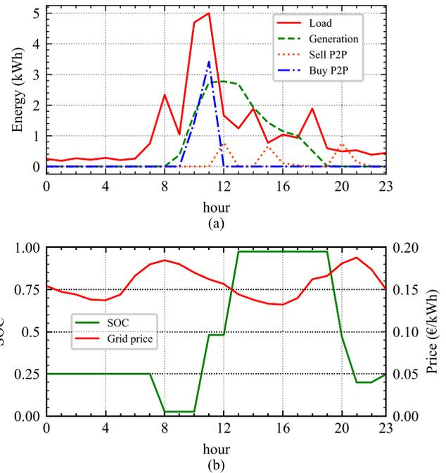
**FIGURE 10.** Evolution of prosumer 1 consumption and energy exchanges (a) and evolution of prosumer 1 SOC and daily prices (b).
