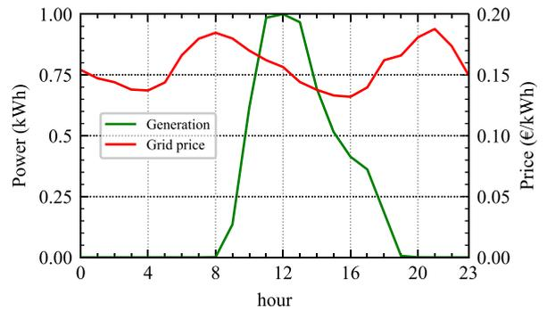
FIGURE 6. Photovoltaic generation profile per unit and day-ahead prices.
