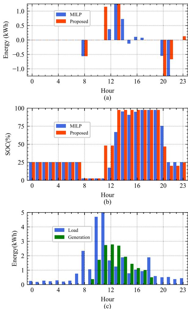
**FIGURE 12.** Evolution of the charge and discharge of the prosumer battery 1 (a), the state of charge (b) with the SoA method and with the proposed method and load-generation profile of prosumer 1 (c).
