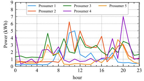
FIGURE 5. Consumption profiles of prosumers.
