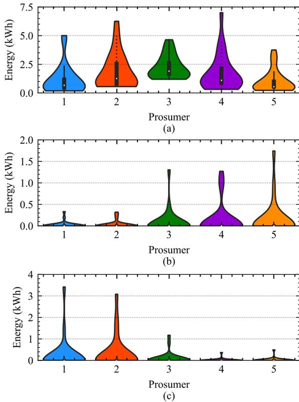
**FIGURE 9.** Violin plot of the consumption of each prosumer (a), the energy purchased from the grid (b) and the energy purchased in the P2P market (c).
