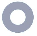
Figure 2.4 Thermal contact area. Inner diameter is 4mm and outer 8mm.
