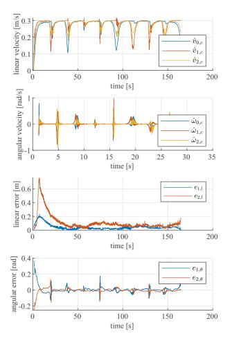
Fig. 6. Linear and angular velocities for a triangular formation of three robots. Target linear velocity:  $0.3\frac{m}{s}$ ; angular velocity limit:  $1\frac{rad}{s}$
