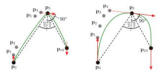
Fig. 2. Demonstration of the usage of two splines while optimizing the curvature of a Beziér-Spline through the control points  $p_1$ - $p_4$
