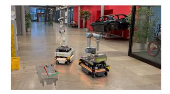
Fig. 7. Triangular formation of three MiR industrial robots. The three robots from left to rigth are: virtual leader, robot 1, robot 2
