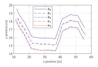
Fig. 5. Target and actual poses for robots 1 and 2 as well as the target pose for the virtual leader.
