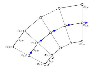
Fig. 4. Target path for a parallel formation of three robots moving in a curve. The equidistant leader path is computed using the aforementioned spline-based planner. The follower paths are derived from the leader path using (9).
