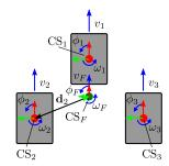
Fig. 3. Overview of a formation containing three mobile robots where each mobile robot is placed with a vector  $d_i$  relative to the formation coordinate system.
