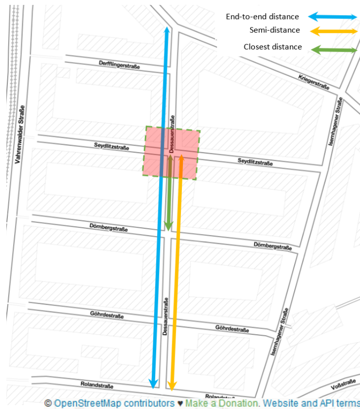
Figure 9. Illustration of the distance-related features of the static model along the north–south intersection approach of a four-way intersection (shown in red).
