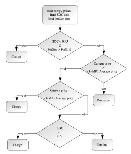
Figure 1. Storage system management scheme for heuristic method.
