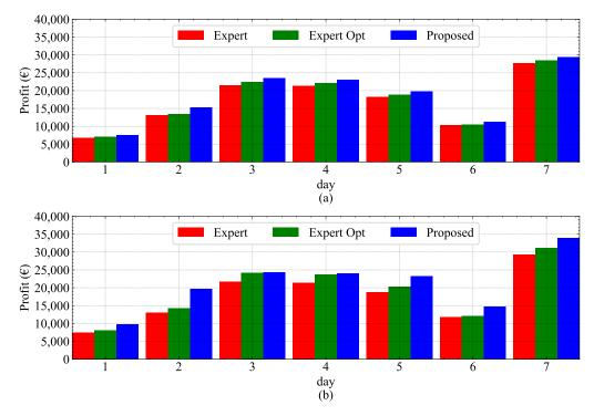
**Figure 9.** Comparison of daily management for case with 100 MW of added generation with 25 MWh of storage (**a**) 75 MWh of storage (**b**).
