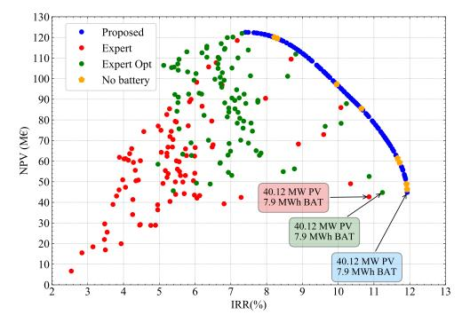
**Figure 10.** IRR vs. NPV for each combination of PV size and battery size using proposed method, expert system and optimised expert system for 30-year investment.
