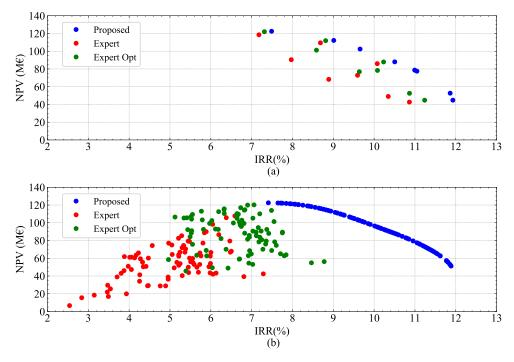
**Figure 11.** Thirty years' investment analysis for each combination, differentiating battery sizes under (a) and over (b) 50 MWh.
