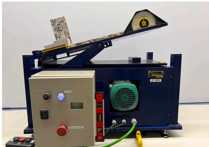
Fig. 3. Tilting system used for the physical models developed at the University of Vigo.
