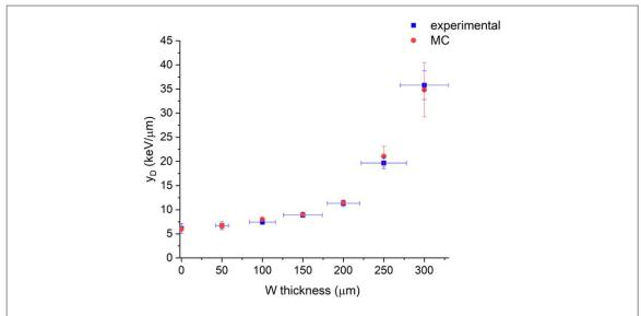
Figure 10. Comparison between experimental and simulated dose-averaged lineal energy  $(\overline{y_D})$  in a silicon 3D-cylindrical microdetector.
