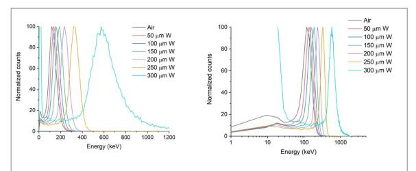
**Figure 6.** Left: pulse height spectra measured by second generation 3D-cylindrical microdetectors as a function of the W foil thickness, corresponding to mean proton beam energies of 13.5, 12, 10.3, 8.4, 6.1, 3.1, 1.9 MeV respectively arriving at the front-face of the SV. Right: Same spectra in a logarithmic scale to easier estimation of the fraction of events into an energy range of interest.
