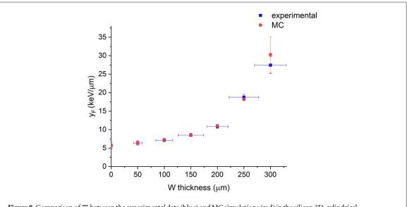
**Figure 8.** Comparison of  $\overline{y_F}$  between the experimental data (blue) and MC simulations (red) in the silicon 3D-cylindrical microdetector.
