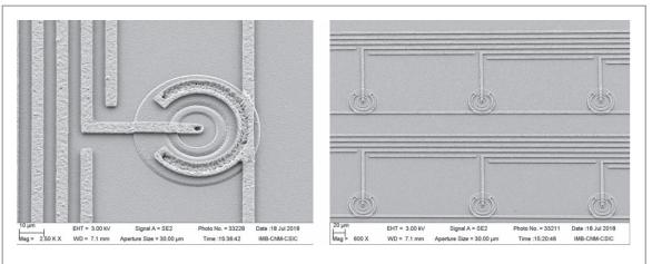
**Figure 1.** Left: SEM image of one second generation 3D-cylindrical microdetector (25  $\mu$ m diameter, 20  $\mu$ m thickness). Right: SEM image of a part of the front-face of the microdetector array with the corresponding metal strips.
