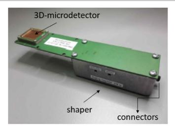
Figure 4. Photograph of the experimental readout-electronics (35 mm  $\times$  170 mm). The 3D-cylindrical microdetector was protected with a kapton layer, which is moved away during the irradiation tests. Connectors consist of 5 V power supply, high voltage power supply for the electronics ( $\pm$ 12 V), and connector for the multi-channel analyzer Amptek MCA8000D.
