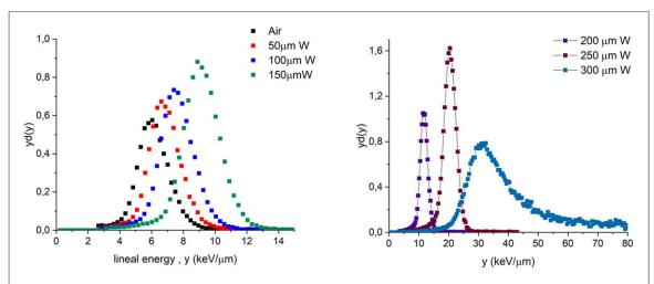
Figure 11. Experimental microdosimetry spectra in a silicon 3D-cylindrical microdetector for different proton energies generated by interposing tungsten foils from 50 to 300  $\mu$ m thickness
