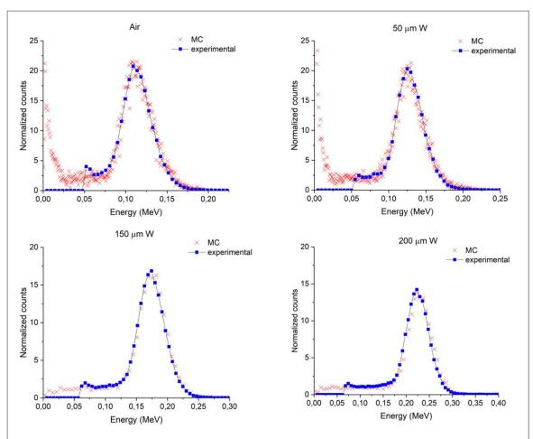
**Figure 7.** Experimental spectra (blue lines) measured with the 3D-cylindrical microdetector and MC simulations (red crosses) for 14.49 MeV protons crossing from 0 to 200  $\mu$ m W foils.
