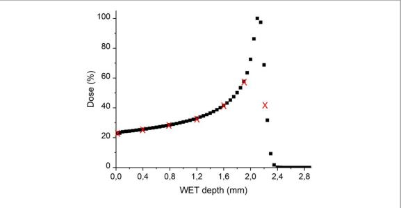
**Figure 5.** Simulated percentage of depth dose curve as the initial 14.49 MeV (0.19 MeV  $\sigma_{\rm exp}$ ) proton beam impinges on a water phantom. Red crosses correspond to the experimental point positions.
