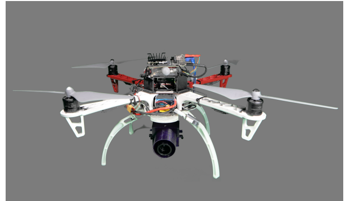
Fig. 3: Aerial robot based on DJI Flamewheel F450 equipped with a DAVIS 346 event camera and a low-cost Waveshare NVIDIA Jetson Nano 2GB Developer Kit used for on-board computation.
