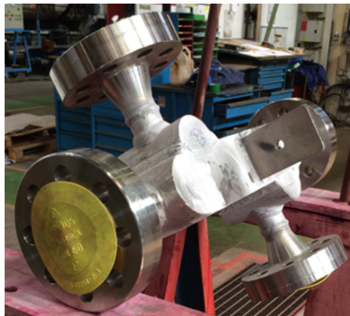
Figure 8. Photo of the SCARABEUS heat recuperator for pure s\text{CO}_2 , designed and manufactured at Kelvion Thermal Solutions laboratories.
