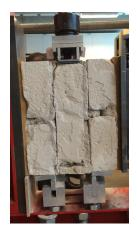
Figure 3. Laboratory shear test on calcium silicate masonry
