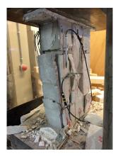
Figure 5. Horizontal compressive test on masonry
