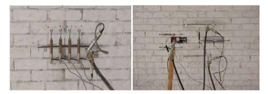
Figure 4. Single flat jack test (left), shove test (right)
