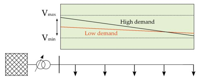
Figure 2. Voltage profile in traditional distribution networks with voltage regulation.
