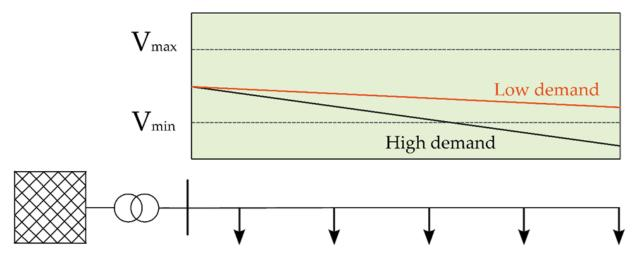
Figure 1. Voltage profile in traditional distribution networks without voltage regulation.
