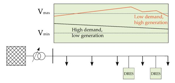
Figure 3. Voltage profile in active distribution networks.
