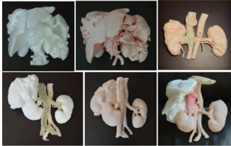
Fig. 2 Discarded models: model 1 (case 1): discarded. Material too stiff for surgery simulation (up, left); model 2 (case 1): discarded. Difficulty to identify the anatomy (up, middle); model 3 (case 2): discarded. Layer thickness too thin (up, right); model 4 (case 3): discarded. Difficulty to assembling parts, high cost and printing time
