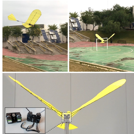
Figure 1. Winged aerial robot built with two servo flapping engines.
