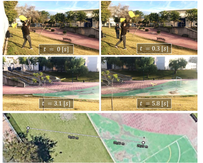
Figure 7. Sequence of images showing the gliding of the winged aerial robot along with the travelled distance.
