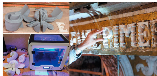
Figure 22. Creation of new volumes in PLA using 3D printing.
