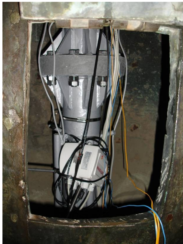
Figure 6. Mounting of sensors inside the "ball" (referred to as sections 1 and 2 in Figure 4.)
