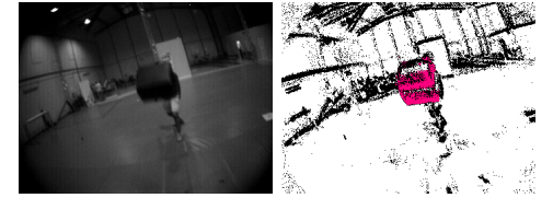
Fig. 4: Event-based dynamic object detection: right) frame from the APS sensor of the DAVIS 346; left) event image of events accumulated during 10 ms (in black) including events detected to belong to the moving object (magenta).
