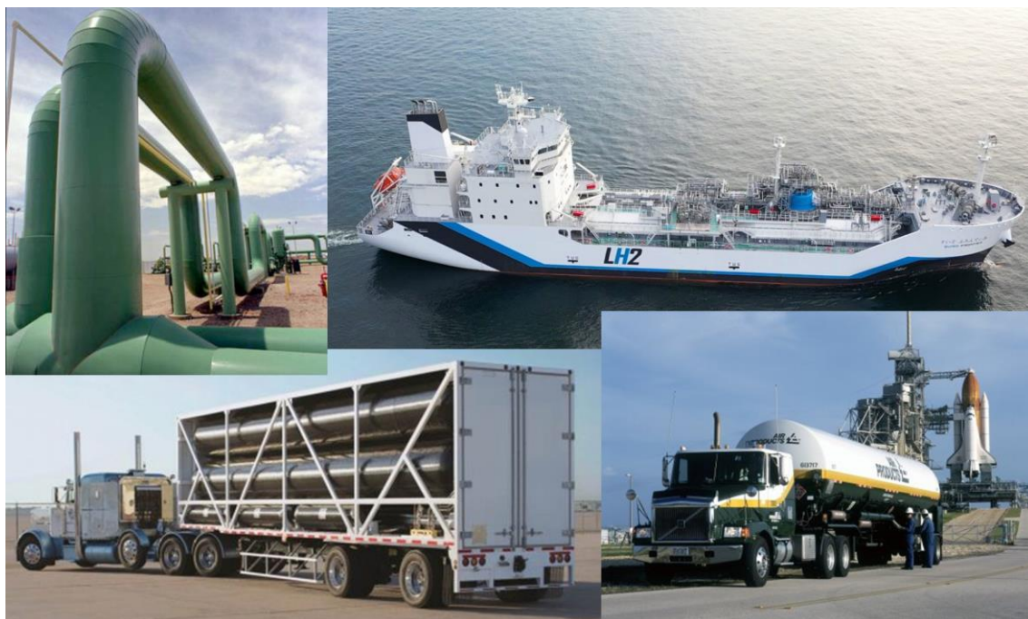
Figure 9. Some of the options for H 2 transportation. Pipelines [33] (upper left), the Suiso Frontier ship [32] (upper right), a tube trailer [27] (bottom left) and a liquid tanker [29] (bottom right)
