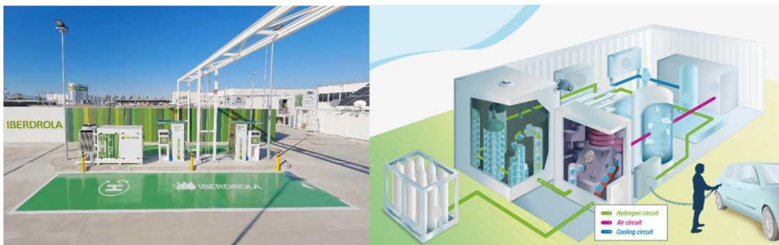
Figure 17. Actual picture [58] and schematic representation of a HRS [59]
