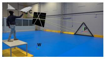
Fig. 3: Diagram of the coordinate frames used by the proposed event-based visual servoing method. C is the camera frame, P is the frame attached to the pattern's plane, and W is the world frame used by the Optitrack system.
