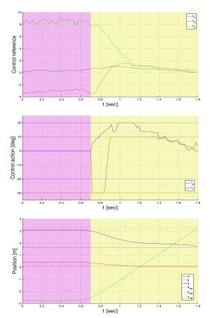
Fig. 7: Evolution of  $\nu(t)$  (top),  $\delta_e(t)$  and  $\delta_r(t)$  (center), and ornithopter 3D positions (bottom) along the maneuver in Figure 5. Purple and yellow colors differentiate between before and after launching. The ornithopter 3D positions were captured by the Optitrack system in the frame W.
