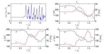
Fig. 5: Top-left) Module of the linear acceleration registered onboard the ornithopter during a guidance experiment. Topright and bottom) Temporal evolution of the Hough  $(\theta, \rho)$  components of the three tracked lines along the experiment. The ornithopter was launched at  $t \approx 0.7$  s.
