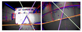
Fig. 6: Line tracking in outdoors under high intensity sunlight (left) and indoor illumination conditions (right). For visualization, the lines are drawn over a frame from the APS along with the events from the DVS.
