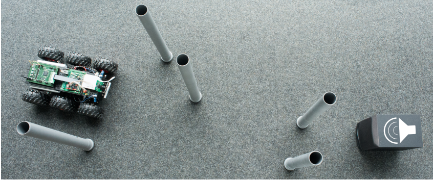
FIGURE 5.14: The autonomous robot navigates through a cluttered environment. It tries to reach a sound source while avoiding obstacles.
