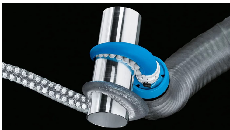
FIGURE 5.1: An octopus-inspired soft robotic arm. Credit: Harvard SEAS.
