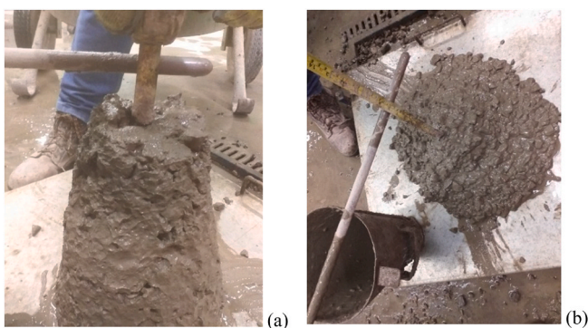
Fig. 18. Slump test for fresh concrete: (a) SCB FA-20 (40 mm); (b) SCB BA-20 (190 mm).
