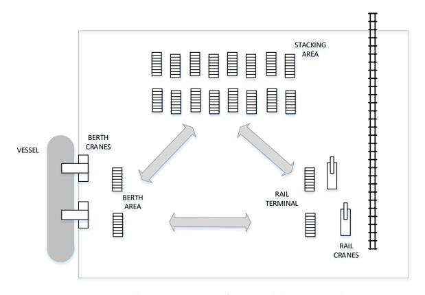
Figure 1. Schematic representation of an intermodal seaport terminal.
