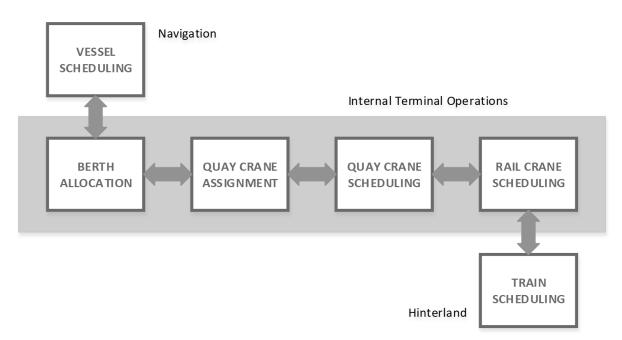
Figure 2. Sequence of planning tasks affecting operations in an intermodal terminal.
