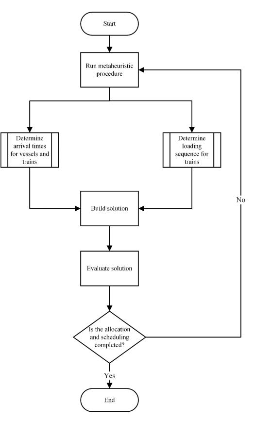
**Figure 4.** Schematic description of the procedure followed to solve the problem using metaheuristic techniques.
