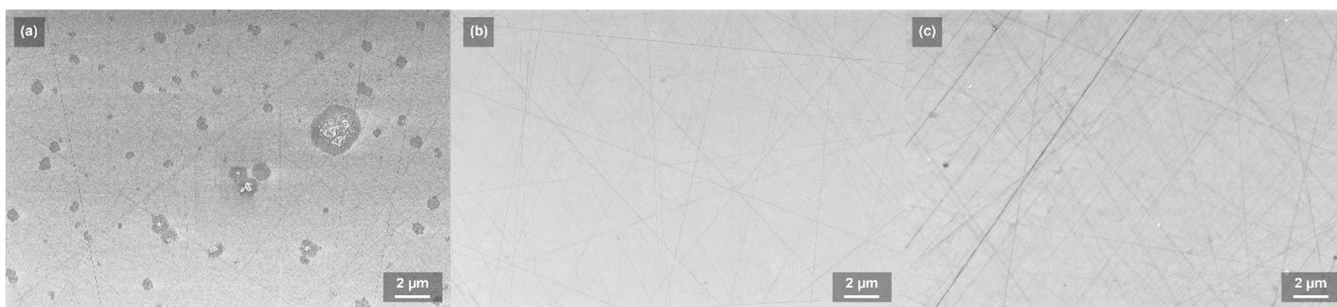
Fig. 5. SEM micrographs of samples produced using "S" sintering schedule from S25CR doped with various concentrations of LiOH (a) additive free, (b) 0.3 wt% LiOH, and (c) 0.6 wt% LiOH.
