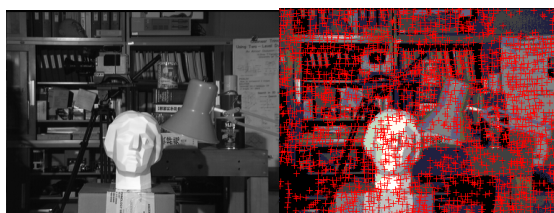
Figure 5: Edge detections in a features-based algorithm.
