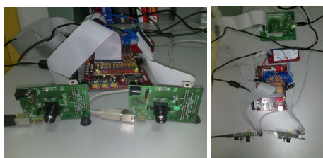
Figure 6: Virtex-5 with AER retinas and USB AERmini2.
