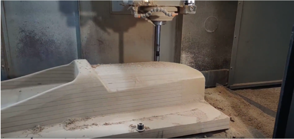
Figure 69: Example of a monocoque positive mold being machined with a CNC, adapted from [35]
