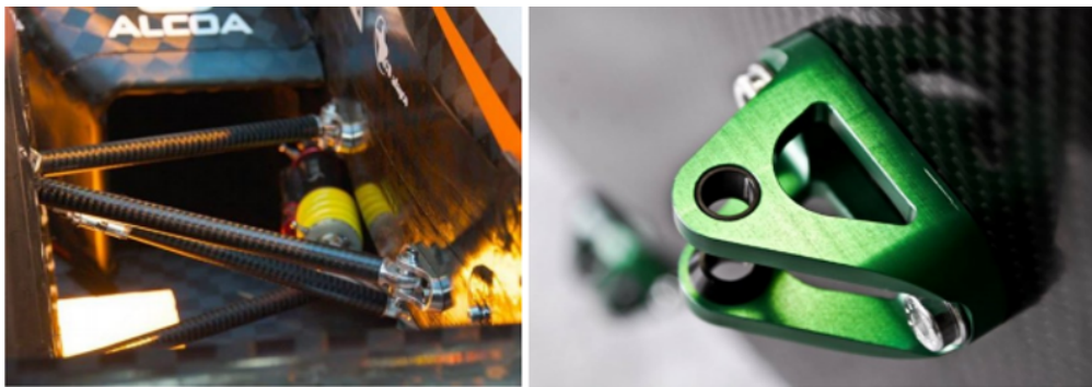
Figure 25: Example of suspension attachment points, adapted from [20]
