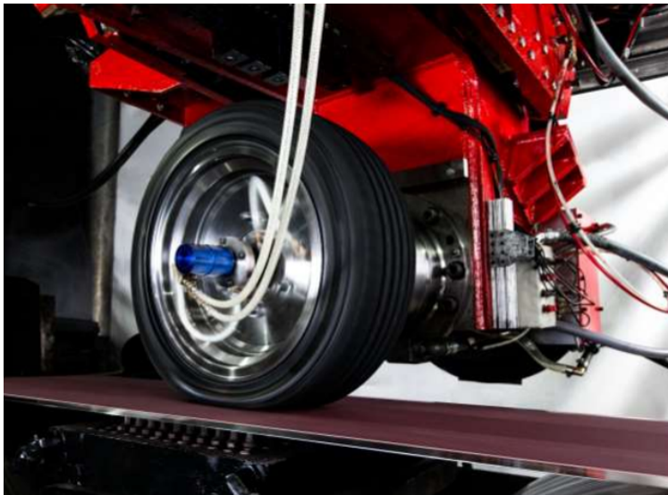
Figure 20: Calspan TIRF tire measurement machine, adapted from [17]
