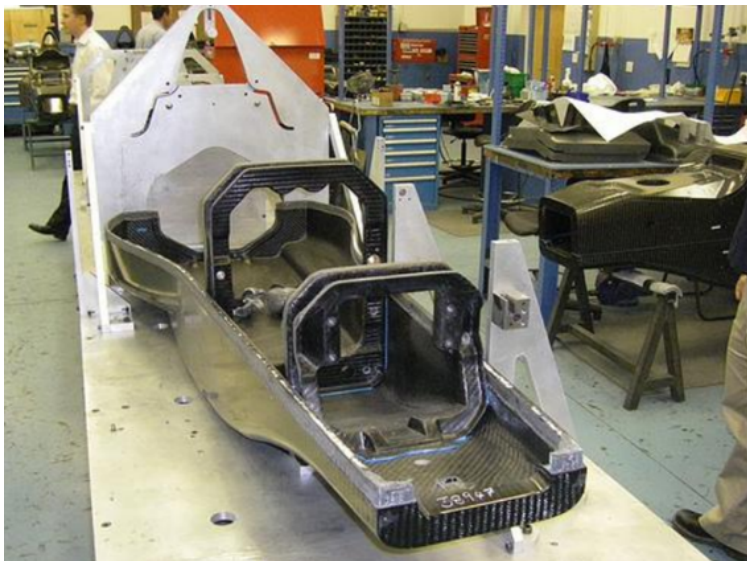
Figure 7: Internal structures inside the monocoque, adapted from[8]
