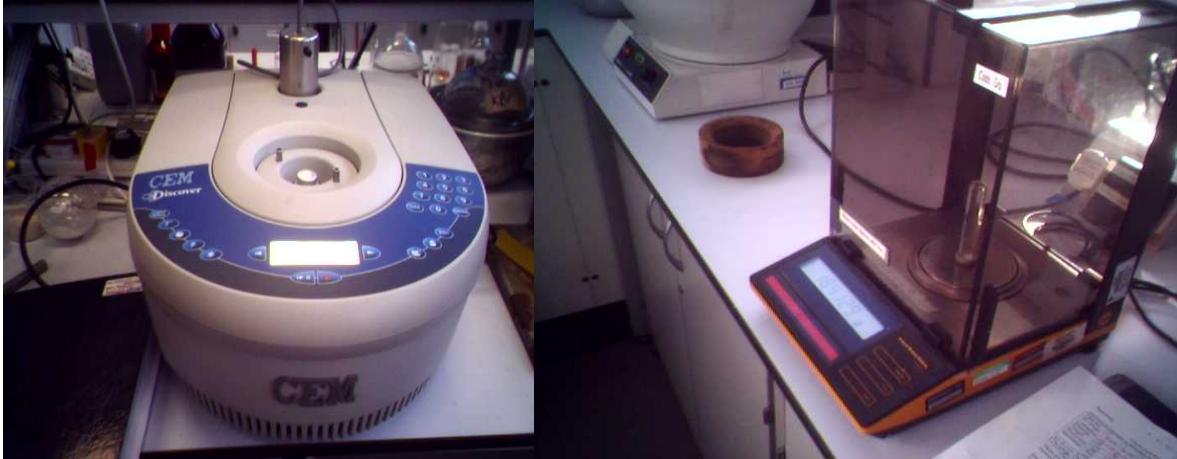
Figure 2: Photograph of the CEM Discover microwave oven with the microwave cavity leakage protection on top centre of the apparatus used .
