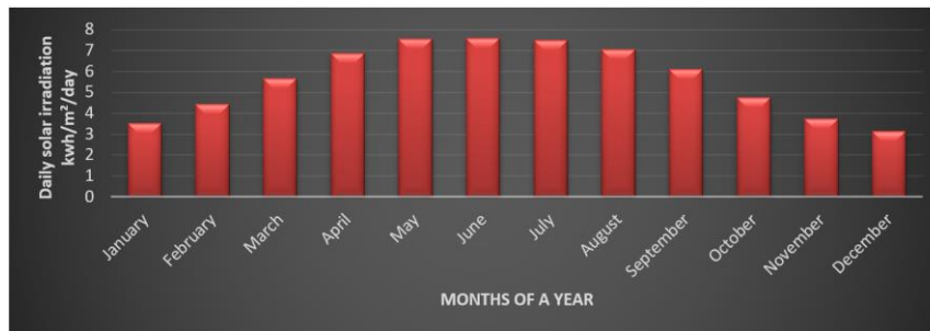
Figure 16. Profile of the average daily solar irradiation and of the brightness index over the course of a year
