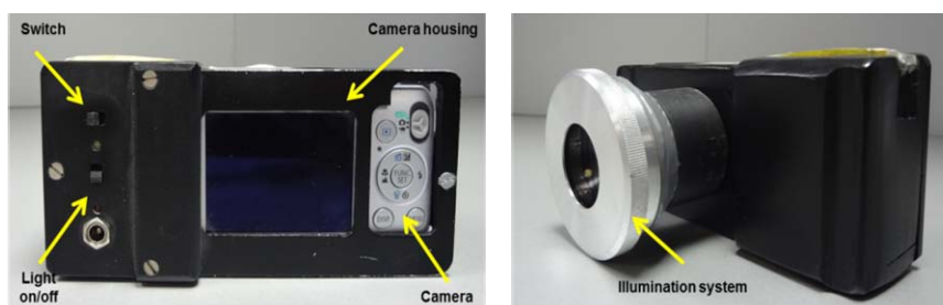
Fig. 2 – Basic operational setup (prototype) for opto-magnetic imaging spectroscopy (NanoLab, Faculty of Mechanical Engineering, University of Belgrade) 12 .
