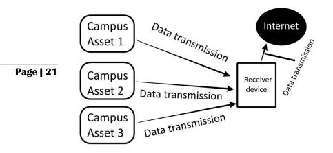
Campus assets may collect measurements and transmit the information to a smartphone or laptop as shown in the figure 1. The cellphone or laptop can analyze the data, such as previous patterns, and notify the user if any metrics exceed the specified limitations. It may also communicate data to the campus's asset management staff through the Internet.
