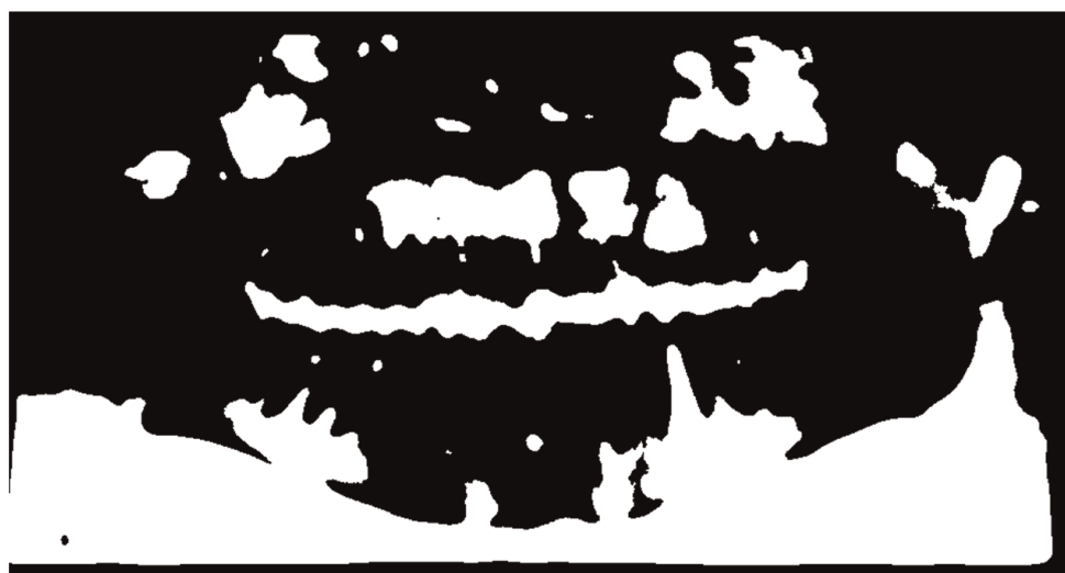
Figure 4. Binarized image using a threshold of 30% from the cumulative function of the histogram of gray levels.
