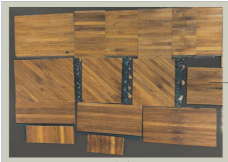
Figure 11. Manufactured bamboo – PLA composite panels (adapted from [36]).
