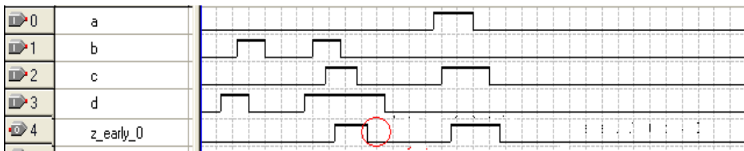
Fig 4.1.11 Early return to 0 appears at output Z (soft error setting hold LUT 011 (1→ 0))
