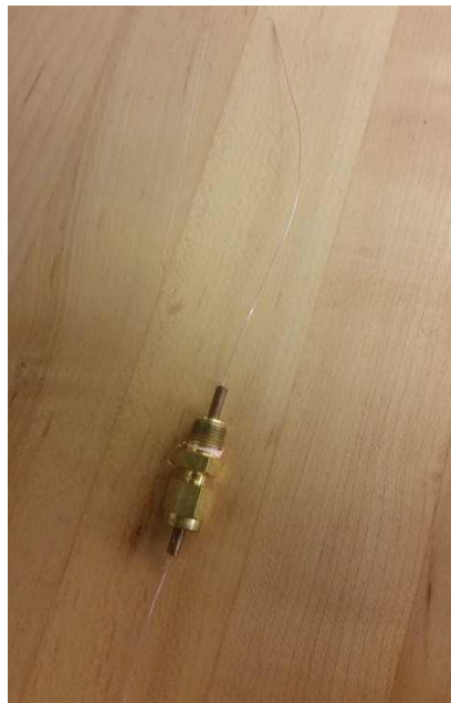
Figure 26. Thermocouple inside the feedthrough and compression fitting.
