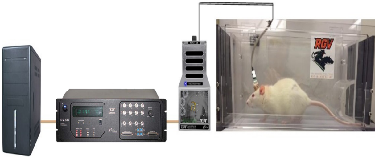
Figure 5.1: The acquisition system setting. One end of a TDT zif-clip digital headstage is connected to a headstage adapter on top of the rat's head and the other end is connected to PZ5 amplifier to boost and digitize the signals
