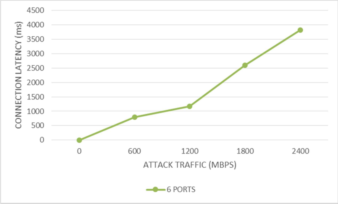
Figure 2.14 The Connection Latency when Smurf attack traffic is sent to all the six ports
