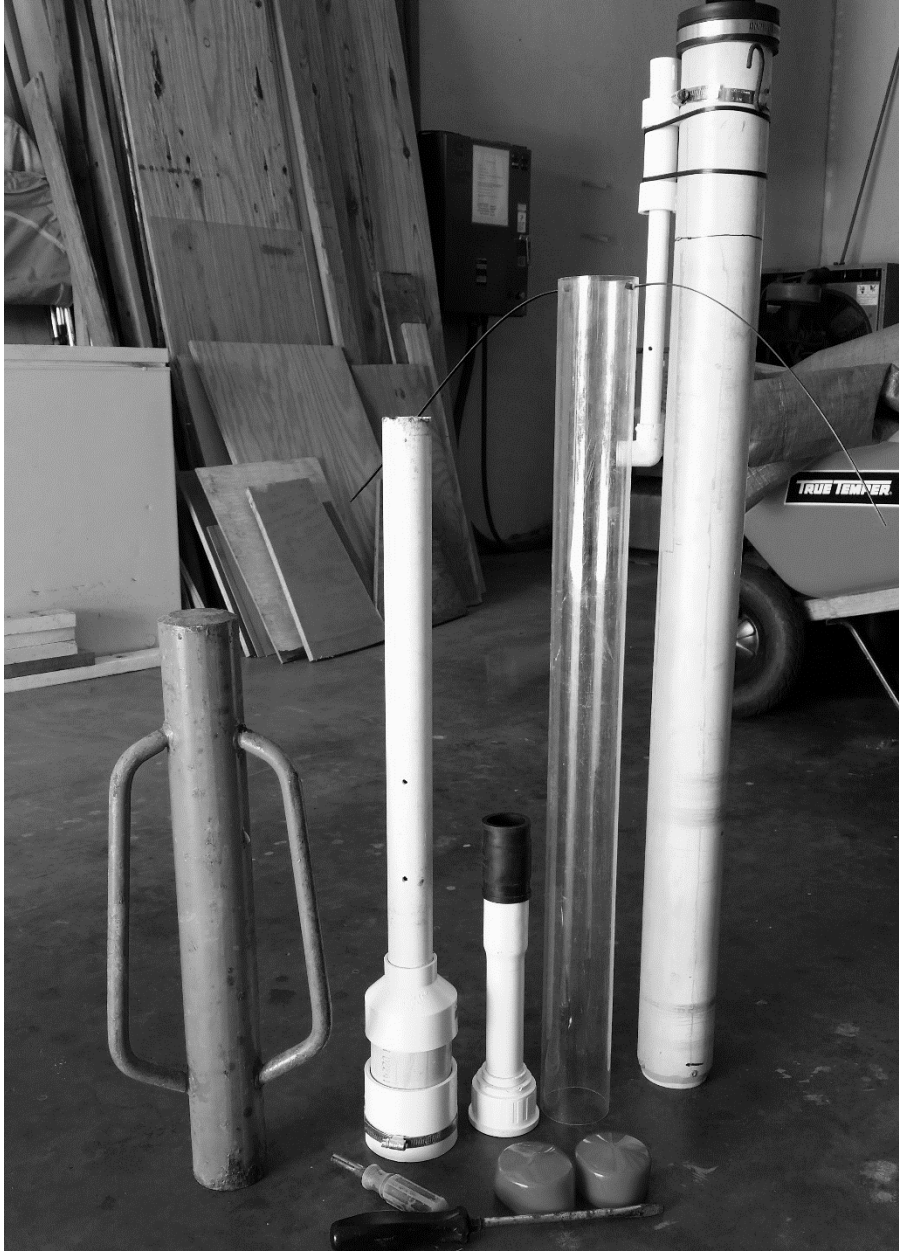
Figure 3: Parts of the sediment corer. The zip ties through the liner are not necessary, but are helpful in pulling the liner free of the corer barrel.
