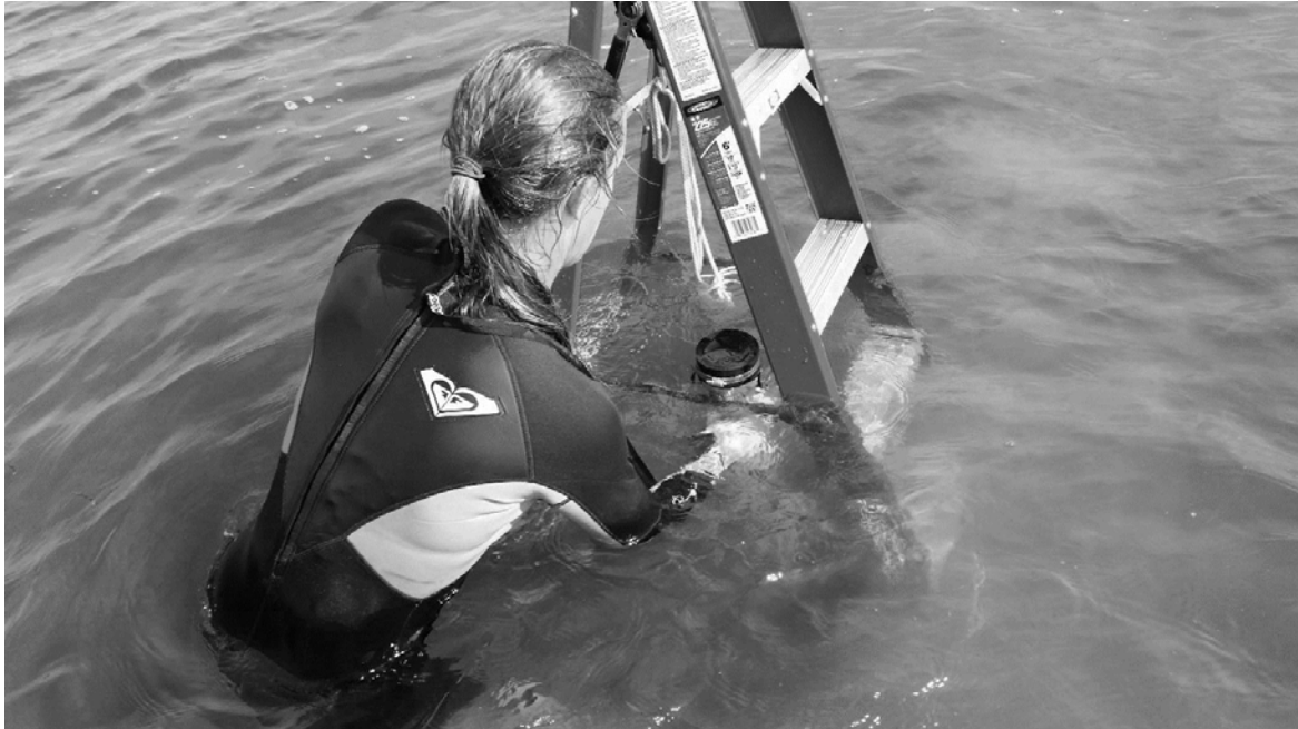
Figure 3: Drawing the core up. The rope seen in the picture was replaced with a length of chain attached to the coring barrel with a hose clamp.
