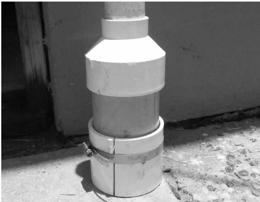
Figure 2: top of the corer. Notice the coupling piece is cut lengthwise so that it is easily removed. All of these pieces are not glued. The interior of the lower coupling tends to crack and the top pipe will become damaged from pounding. Not gluing them makes them easily replaceable.
