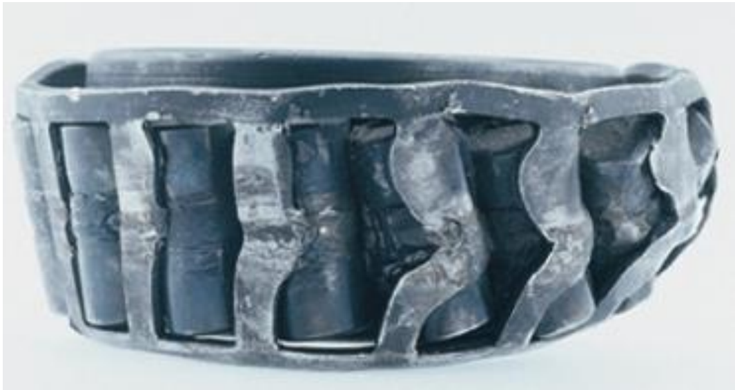
Figure 1.5. Level 4 – Total Bearing Lockup
