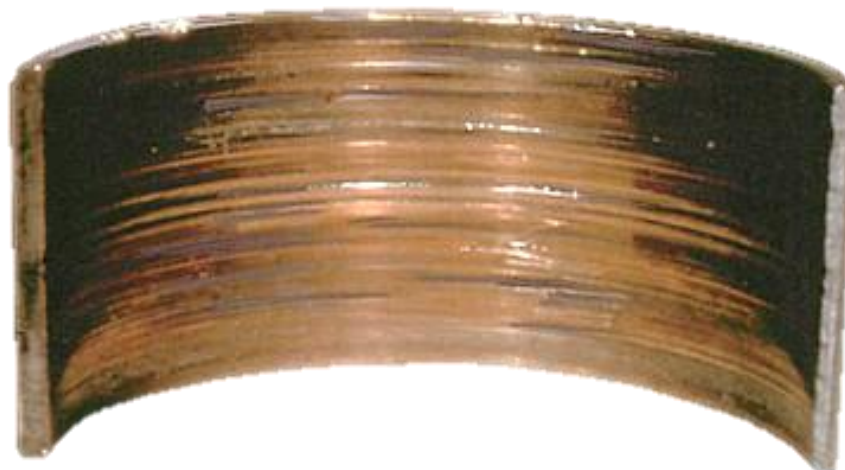
Figure 1.3. Level 2 – Scoring and Peeling
