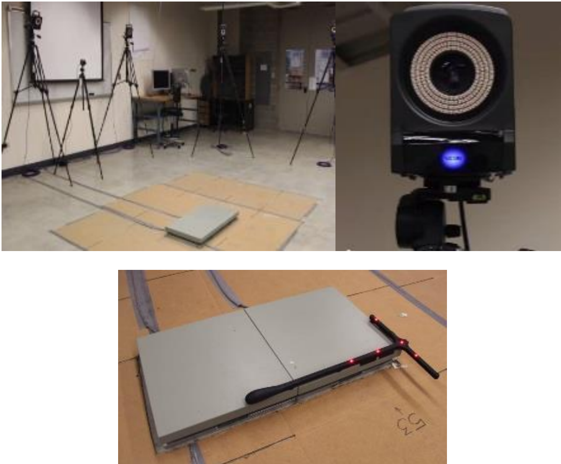
Figure 4.6 Biomechanics Laboratory at UTPA, NSF grant (Left), Vicon Motion Analysis System camera (Middle), and Force Plates (Right).
