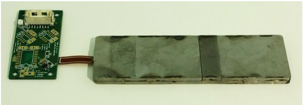
Figure 17: Aluminum Heatsink Used for Welding
