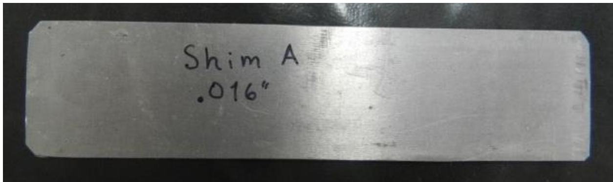
Figure 25: Shim A, 0.016 Inch Thick Aluminum Sheet
