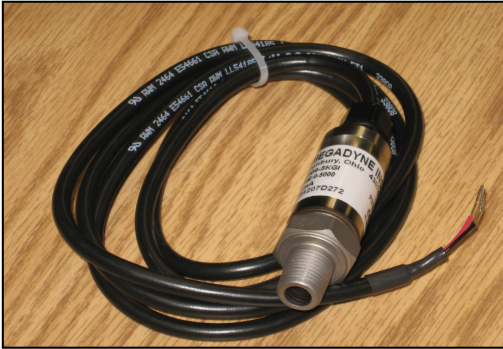
Figure 32: A picture of the PX 309-5KGI pressure transducer model.
