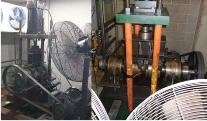
Figure 2. Photographs of the dynamic bearing testers used to conduct the experiments for this study.
