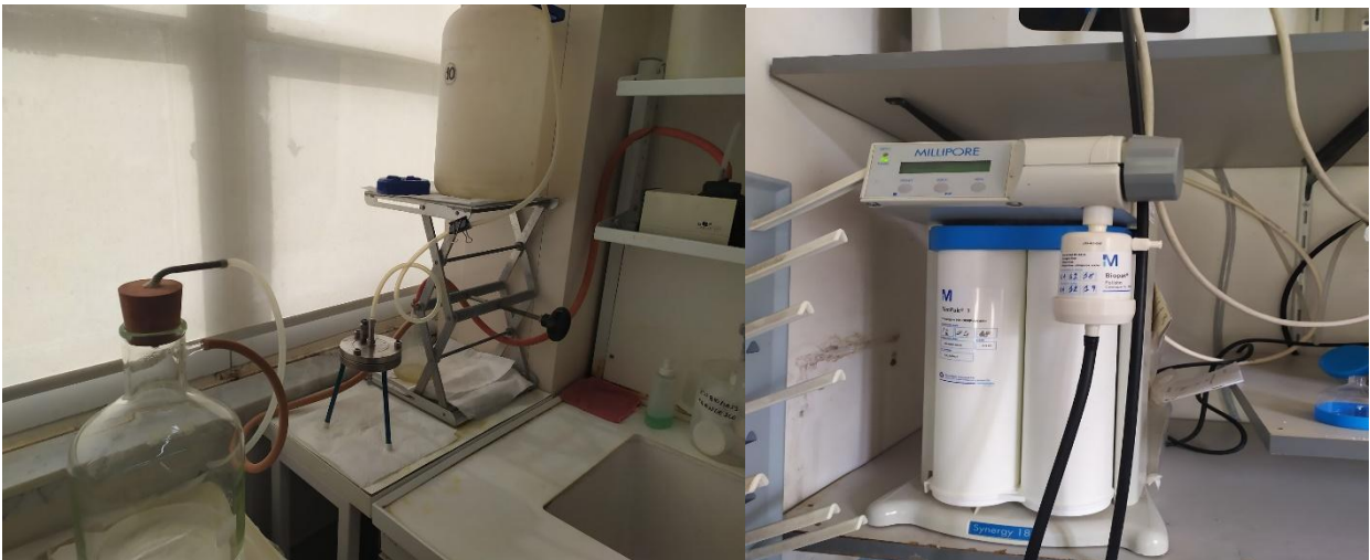
Figure M1. Sea water filtration assemblage (left); Millipore filtration apparatus (right). The water is collected in the Schott DURAN 10L glass carboy with vacuum adapter.
