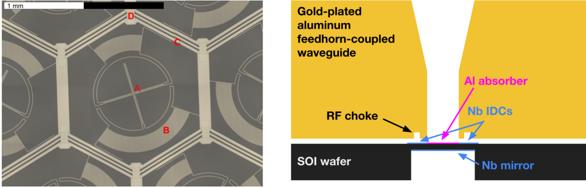
Fig. 1. Left : Image of an 220 GHz pixel, consisting of two orthogonally aligned inductors (A) coupled to arc-shaped IDCs (B), which are in turn coupled to the coplanar waveguide (CPW) feedline (C). The CPW is bridged at the six vertices of each hexagonal pixel cell (D) to maintain ground-plane connectivity. This device is aluminum-only, but on final devices, structures B, C, and D will be made out of niobium. Right : Diagram taken from [12], showing the pixel's position beneath the feedhorn-coupled waveguide and above the integrated silicon quarter-wavelength optical backshort.
