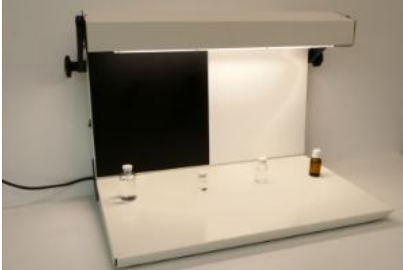
Figure 2.2. Apollo II Liquid Viewer Station
