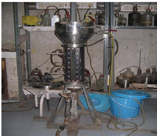
Fig. 1. (a) Experimental Set-up of anoxic HR, (b) Nitrifying granules in aerobic HR.
