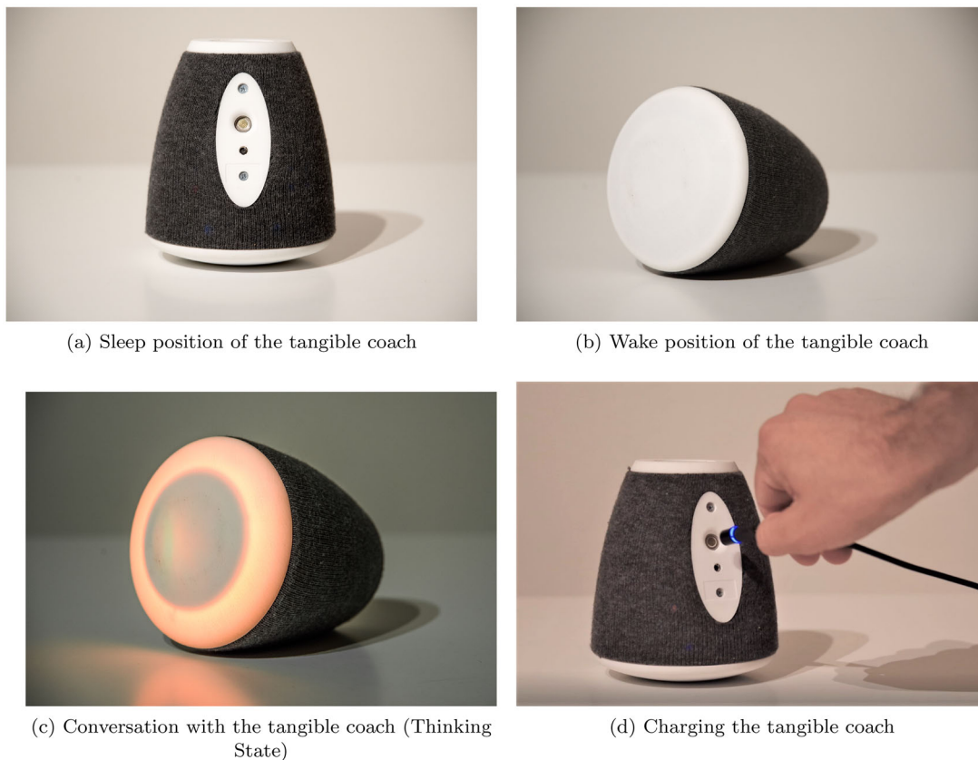
Figure 13. Different states. (a) Sleep position of the tangible coach. (b) Wake position of the tangible coach. (c) Conversation with the tangible coach (Thinking State). (d) Charging the tangible coach.
