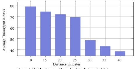
Figure 4-16. The Average Throughput vs Distance in bits/s
