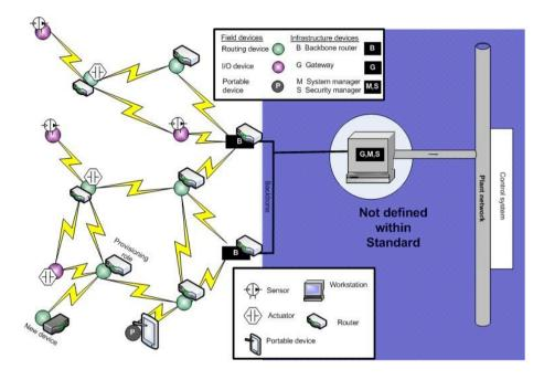
Figure 2-6. ISA.100 Network Architecture adapted from [67]
