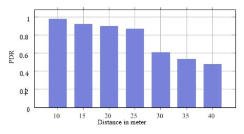
Figure 4-15. Packet Delivery Ratio vs distance
