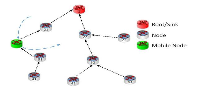
Figure 3-2. Static WSN with Mobile Node
