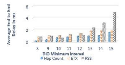
Figure 4-29. The Average End-to-End Delay vs DIO Minimum Interval
