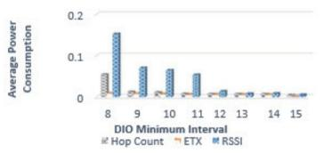
Figure 4-28. The Average Power Consumptions vs DIO Minimum Interval in mw
