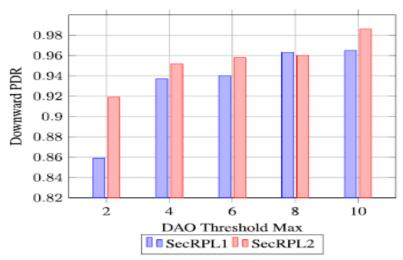
Figure 4-52. Downward PDR under Various DAO Threshold
