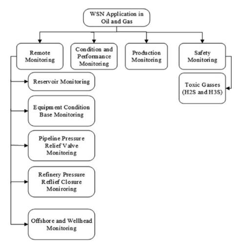
Figure 2-1. Classification of WSN Applications in Oil and Gas Industry [41]
