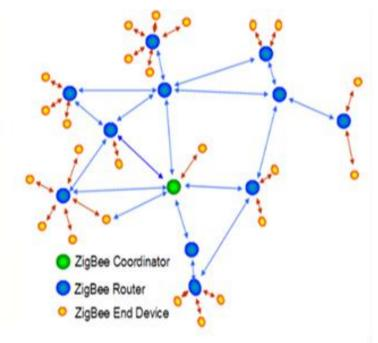
Figure 2-4. ZigBee network [60]
