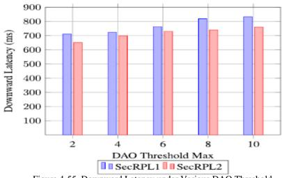
Figure 4-55. Downward Latency under Various DAO Threshold
