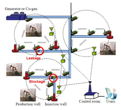
Figure 2-2. Oil Distribution and Monitoring using WSN [49].
