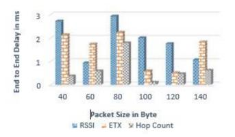
Figure 4-27. The Average End-to-End Delay vs Packet Size
