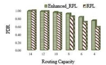
Figure 4-32. The Packet Delivery Ratio of RPL and Enhanced-RPL in Grid Topology
