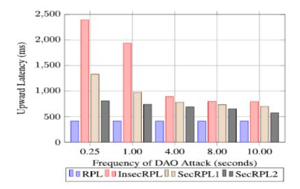
Figure 4-40. Upward Latency vs Attack Intervals
