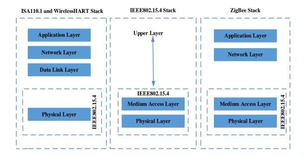
Figure 2-7. Protocol Stacks of ISA100.11 A, WIRELESSHART, IEEE802.15.4, AND ZIGBEE [68]
