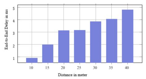
Figure 4-17. The End-to-End Delay vs Distance in m/s
