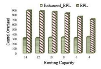
Figure 4-34. The Control Overhead of RPL and Enhanced-RPL in Grid Topology
