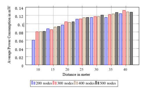
Figure 4-18. Power Consumption vs Distance for Different Node Number in mW
