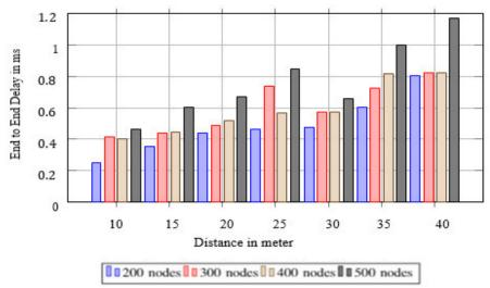
Figure 4-21. The End-to-End Delay vs Distance vs for Different Node Number
