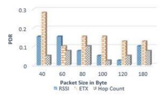
Figure 4-25. The Average Packet Delivery Ratio vs Packet Size
