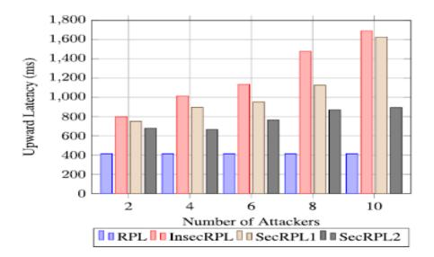
Figure 4-46. Upward Latency vs Number of Attackers
