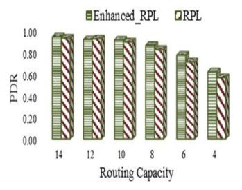
Figure 4-35. The Packet Delivery Ratio of RPL and Enhanced-RPL in Random Topology
