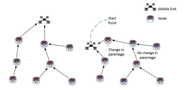
Figure 3-3. WSN with Mobile Sink Node
