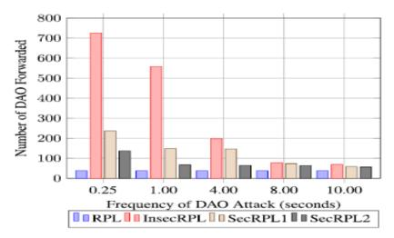
Figure 4-38. DAO's Forwarding Overhead vs Attack Intervals
