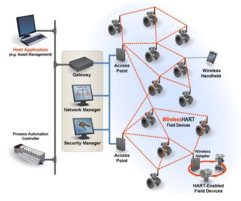
Figure 2-5. WirelessHART Network Architecture adapted from [60]
