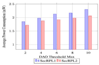
Figure 4-51. Power Consumption under Various DAO Threshold
