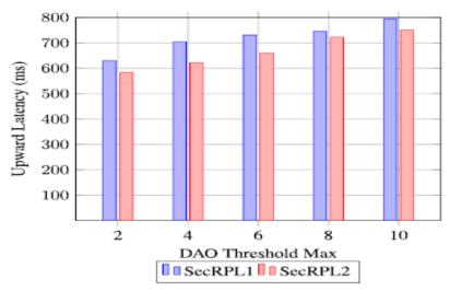
Figure 4-54. Upward Latency under Various DAO Threshold
