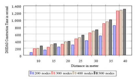
Figure 4-22. DODAG Construction Time vs Distance for Different Node Number
