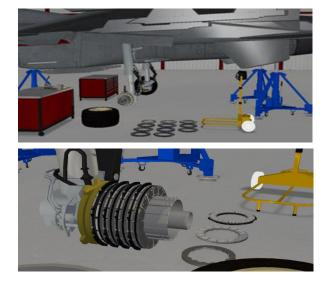
Fig 3. Disassembly of the wheel and brake disks
